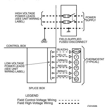
Fig. 2—48GP High- and Control-Voltage Connections
